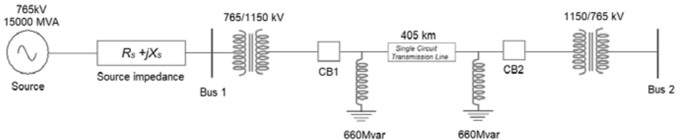
Fig.1 Schematic of 1200kV UHVAC system
