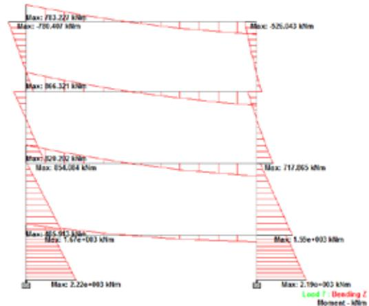
Fig 11. Bending Moment Diagram
