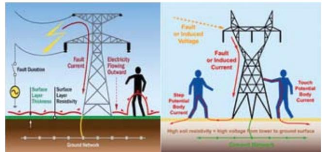
Fig.2 Step and Touch Potential During Fault
