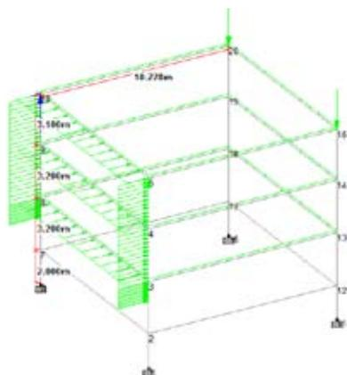
Fig 10. Uplift and compression loads pedestals in Vertical direction
