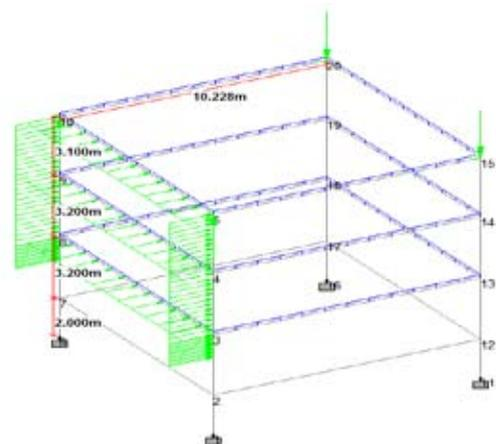
**Fig 7.** Vertical loads on beams
