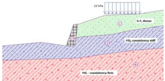
**Fig 16:** Typical slope stability study assignment
