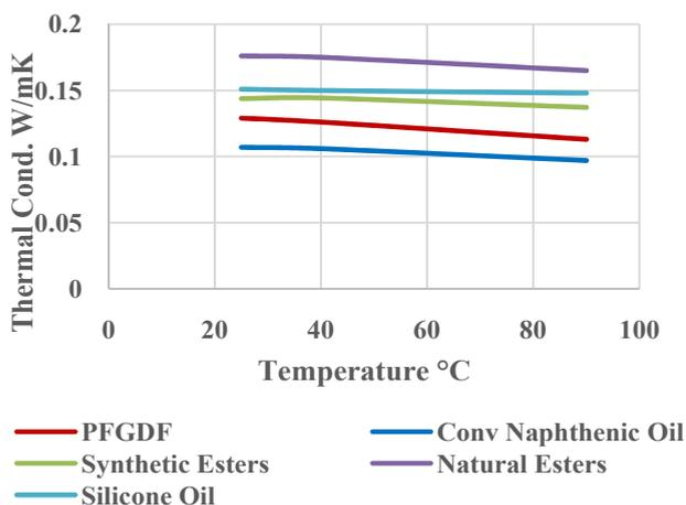
Fig. 3: Thermal conductivity of DFs
