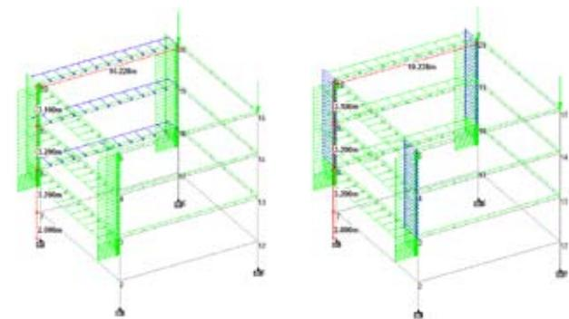
Fig 9. Horizontal loads on beams and pedestals in diagonal direction
