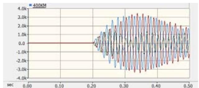
Fig 2: Overvoltage waveform when no control is used
