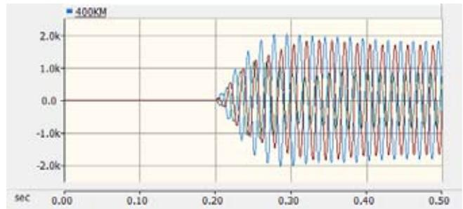
**Fig 6:** Overvoltage waveform when both PIR and Shunt Reactor is used
