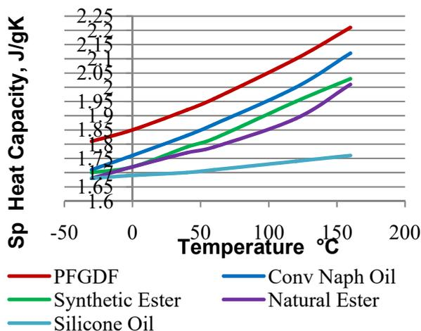
Fig. 4: Specific Heat Capacity of DFs
