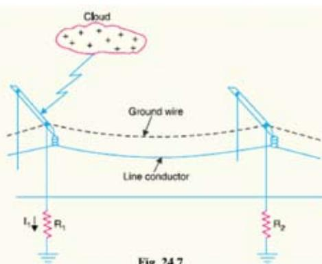
Fig.4 Lightning Strike on Transmission Line
