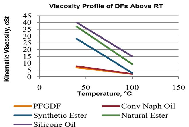
Fig. 2: Viscosity Profile of DFs
