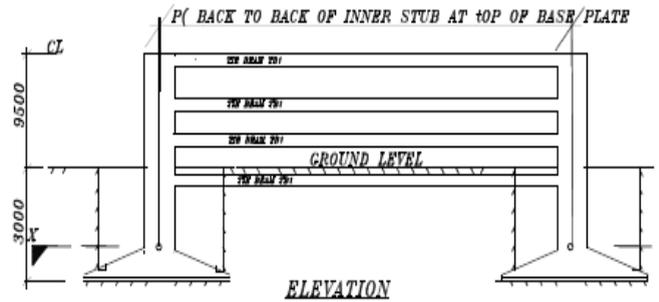
Fig 17. Typical Elevation of foundation showing tie beam arrangements
