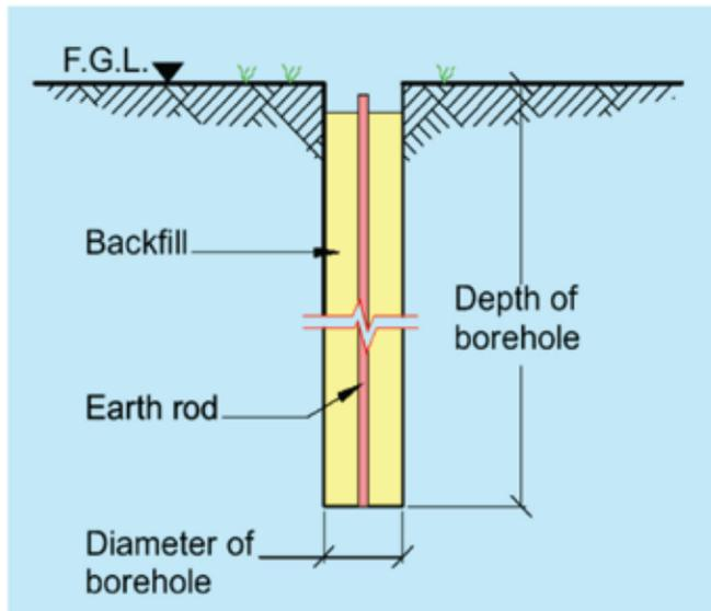
Fig 7 Concept of Chemical Grounding
