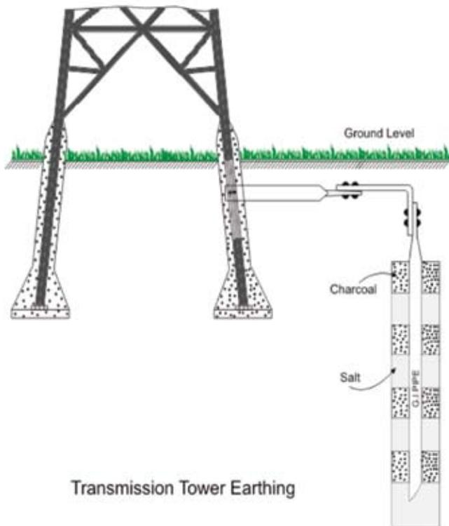
Fig 9 Transmission Tower Grounding (Treated)
