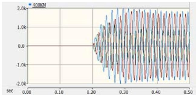
**Fig 4:** Overvoltage waveform when only PIR is used
