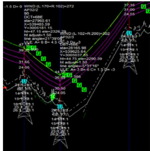
Fig 14: Tower 91 with leg extension
