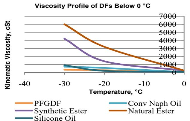
Fig. 1: Viscosity Profile of DFs
