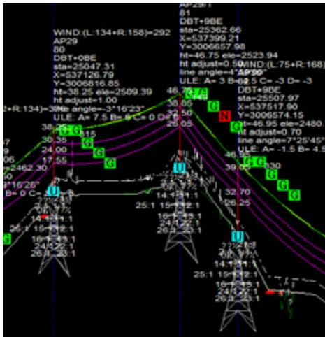
Fig 15: Tower 81 with leg extension
