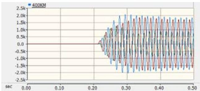
Fig 8: Overvoltage waveform when PIR with controlled switching and shunt reactor is used
