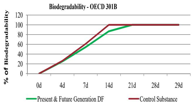
Fig. 9: Biodegradability Curve
