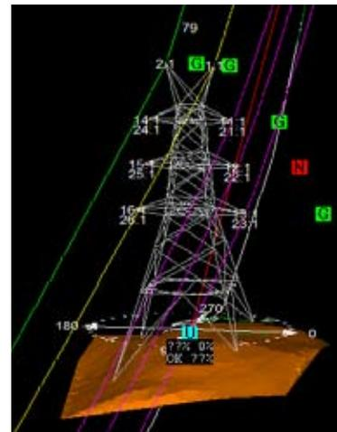
Fig 10: Tower at location number 79 with leg extensions on TIN ground profile
