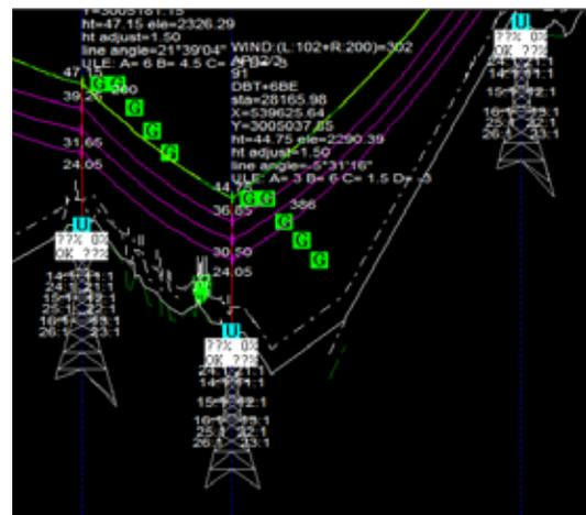
Fig 14A: Tower at 81 without leg extension
