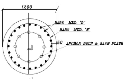
Fig 16. Typical Cross Section of Pedestal
