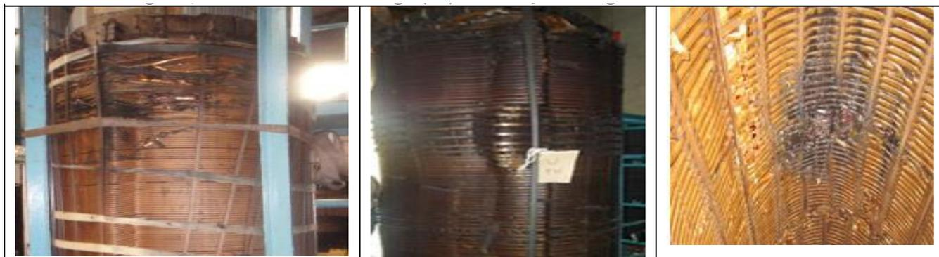
**Fig. 3 :** Failures in Low Voltage (LV) / Tertiary winding due to inter turn short
